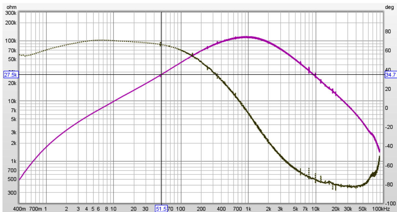
Figure 8. Primary winding impedance of WWFB with 8.5Ω secondary configuration.
