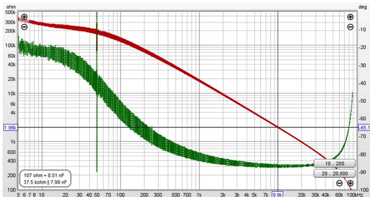
Figure 14. Shorted primary to shorted secondary impedance for WWFB
