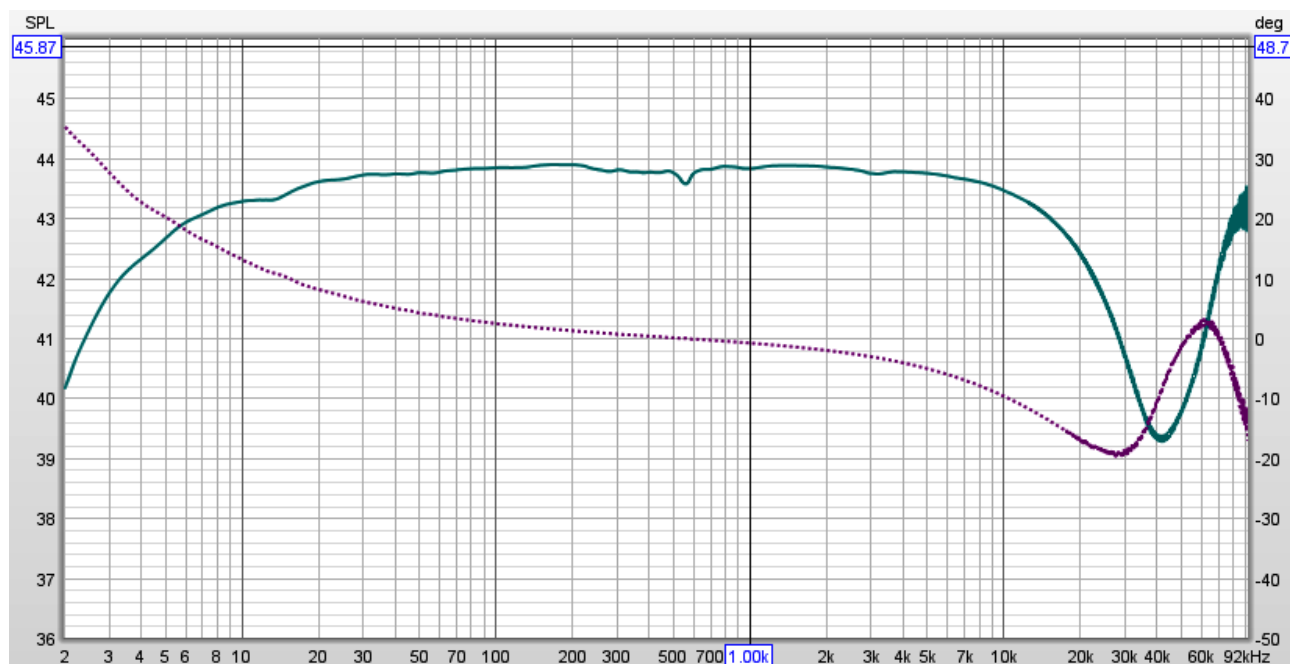
Figure 25. Frequency response of AF8/2 with 2Ω secondary configuration and load
