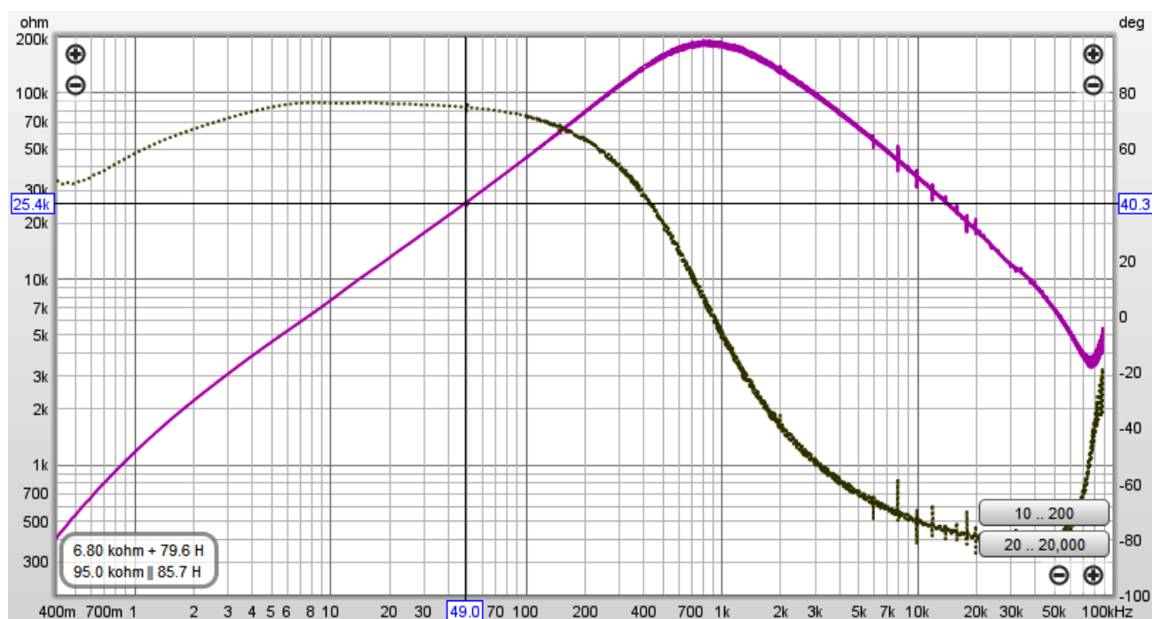
Figure 9. Primary winding impedance of Ferguson OP25 (new) with 4Ω secondary configuration.
