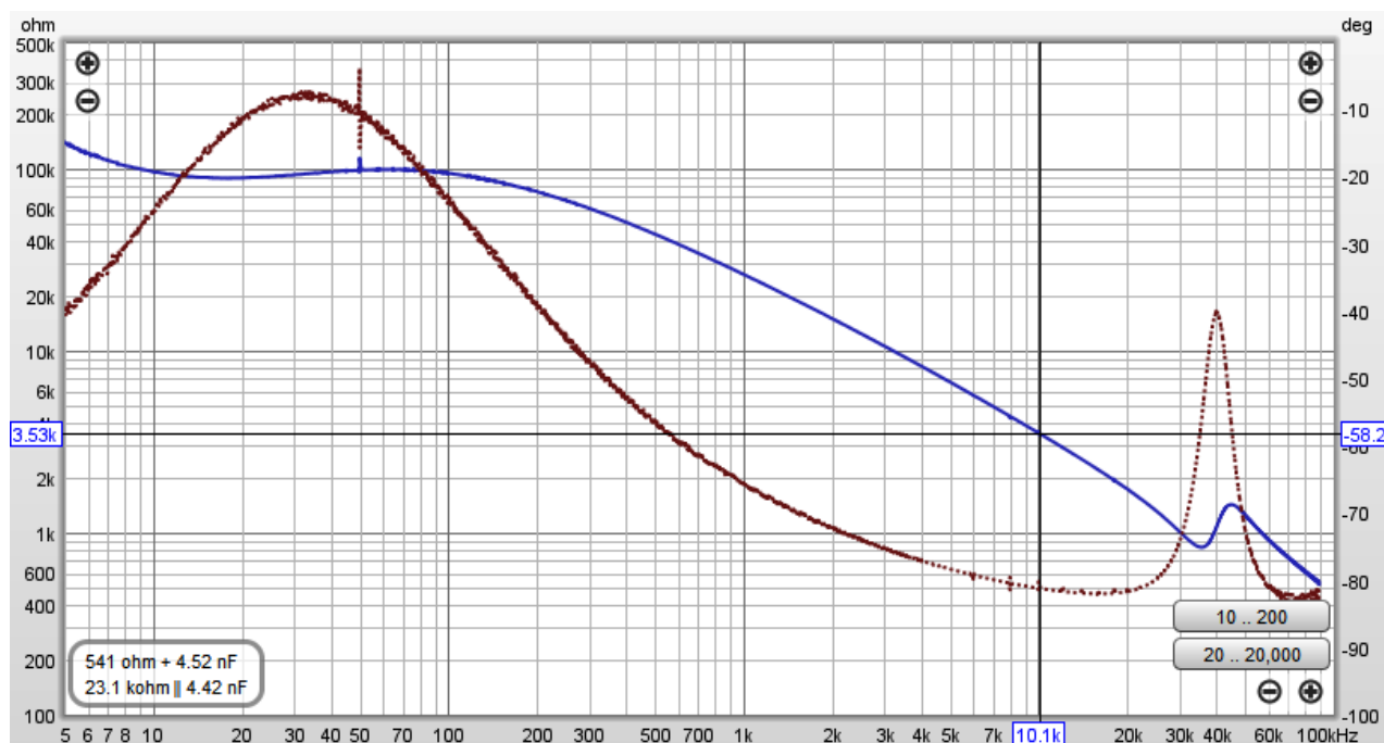
Figure 16. Shorted primary to shorted secondary impedance for Ferguson OP25/15 (new)
